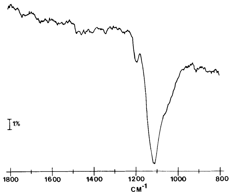
FIGURE 7 Infrared spectrum of \gamma -glycidoxypropyltrimethoxysilane adsorbed onto aluminum from catalyzed 1% aqueous solution.
